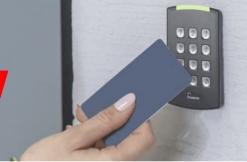
Intrinsically linking the security systems provides solutions to applications that are not possible using separate access control and intrusion systems. Presentinga card at a reader for example, will disarm the area behind the door (if theuser is authorized to do so) and automatically unlock the door once the areais disarmed.
